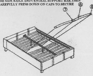
STEP 5 ATTACH THE METAL TIE-ROD (N) IN THE CENTRE OF THE BED INTO PRE-DRIL LED HOLES IN THE SLAT SUPPORTS, SCREWING ROD TO SUPPORTS WITH I, J, K & L ONCE ROD IS FIXED IN POSITION, STICK RUBBER PAD (M) TO TOP OF THE METAL CENTRE SUPPORT, DIRECTLY UNDER THE TIE-ROD SO THERE IS NO CONTACT BETWEEN SUPPORT & ROD.
